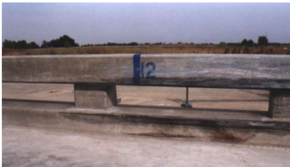
Figure 2-21 Post Impact Bridge Rail Scuff Marks Test 544
