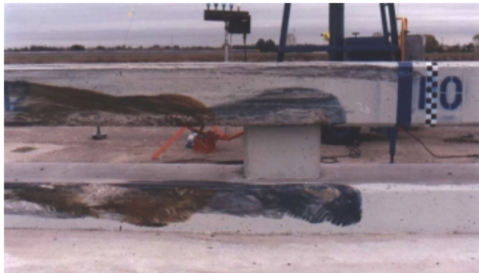
Figure 2-31 Test 545 Impact Area
