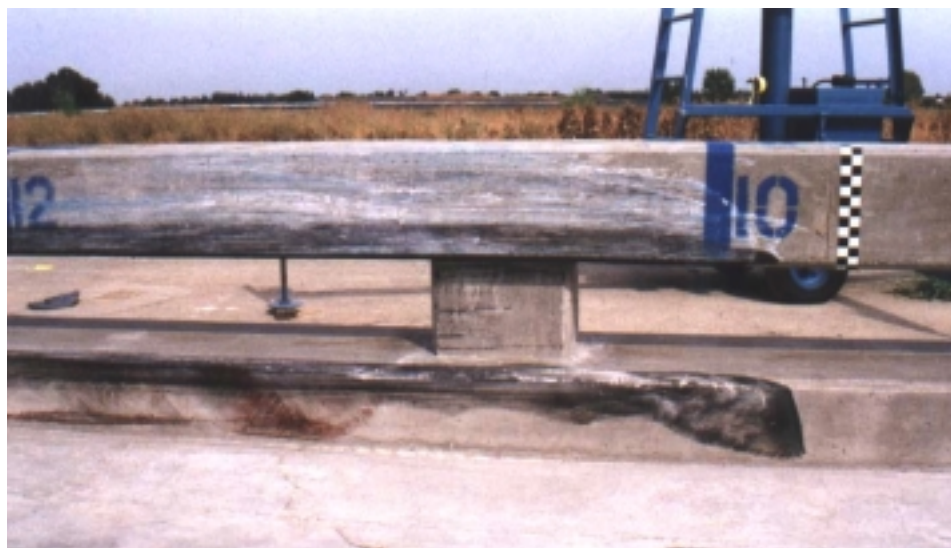
Figure 2-20 Post Impact Bridge Rail Scuff Marks Test 544
